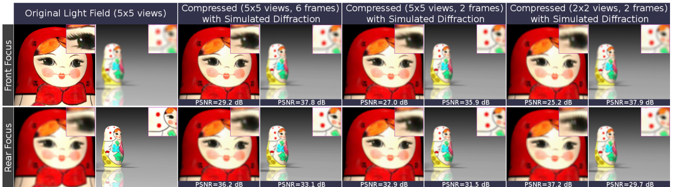
Fig. 10. Simulated retinal blur and diffraction. Images show closeups of close and far matryoshka dolls from the light field shown in Fig. 3, and inset images show further magnification. The larger doll is virtually positioned at 17 cm in front of the display and the rear doll at 18 cm into the display. The views of the light field are evenly spaced over a pupil of a = 5 mm for a single eye, with the outermost views centered at the pupil edges. Compressed images reflect the configuration of our prototype display: 1 LCD layer in front of a HARB, a f = 31.8 cm focal length lens, a viewing distance of d_e = 127 cm, and native panel resolution of 39.1 cycles/degree at this distance. Diffraction is approximated using the method described in Section 3.5 using the wavelengths \lambda_{red} = 700 nm, \lambda_{green} = 546 nm and \lambda_{blue} = 435 nm. Rows: Synthetically refocused images of front doll ( first rows ) and rear doll ( second rows ). First column: Source light field. Following three columns: Compressed version of the source light field using the decomposition algorithm described in Section 3.1.2 in the noted configurations. High quality retinal blur can be achieved in the presence of diffraction ( second column ), but quality suffers if compression is too high ( third column ) or angular resolution is too low ( fourth column ). Matryoshka doll model by artist “coiboide” of Turbosquid.com.
