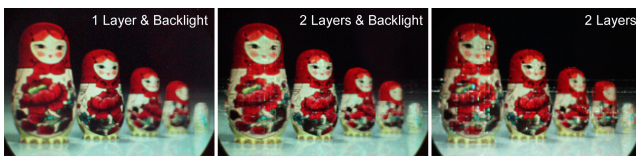
Fig. 14. Failure case photographs for dual layer architectures. In practice imprecise alignment of prototype layers creates artifacts. Artifacts are also observed in simulation, as narrow view spacing poses a challenge for large LCD pixel sizes. Matryoshka doll model by artist “coboide” of Turbosquid.com.
