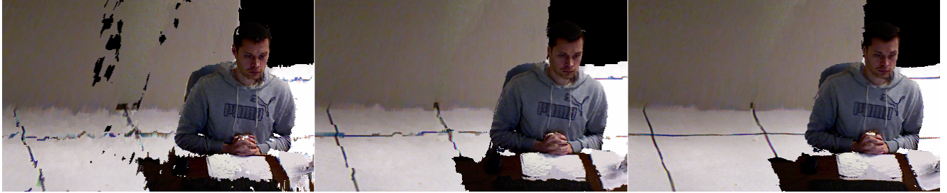
Figure 14: Smoothing results. Left: No smoothing (or hole filling) applied. Center: Median smoothing. Right: Bilateral smoothing.
