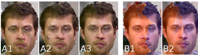
Figure 15: Data merger results. A1: No merger applied, meshes drawn on top of each other. A2: Merger with simple average. A3: Merger with quality weighting. B1: Color coded camera contributions with no merger. B2: Camera contributions with quality-weighted merger.
