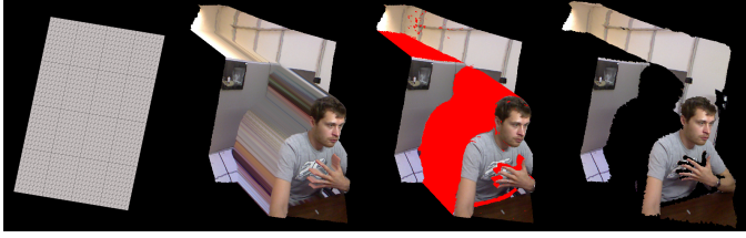
Figure 8: Fast Meshing for the Kinect. Left: Triangle mesh template stored in GPU memory. Center-Left: Vertex shader extrudes template using camera intrinsics and depth texture. Center-Right: Geometry shader rejects triangles corresponding to missing or discontinuous surfaces (shown in red). Right: Resultant textured mesh.
